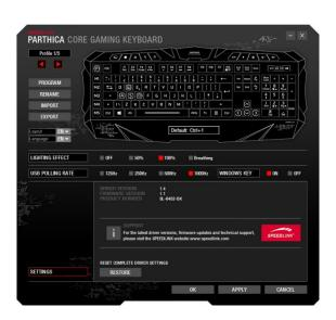
In the index tab "Settings" you can see the driver version, firmware and article number. Note below which refers to our support team. With the button reset you can perform a hardware reset.
