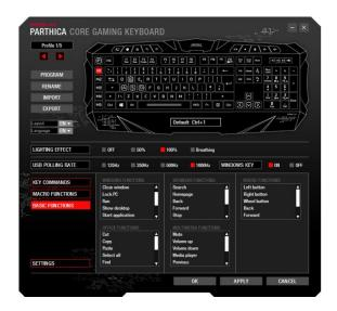
Advanced basic and mouse functions can be assigned to macro-capable buttons: Choose the desired function and confirm by clicking "APPLY".
